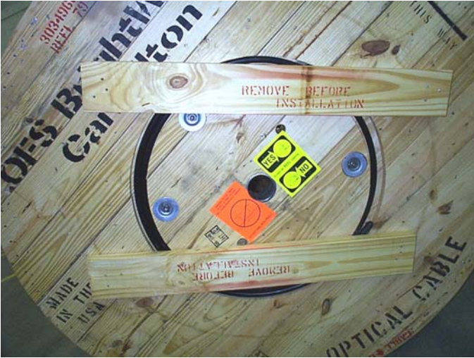
Figure 1 - Protective wood lagging boards.
